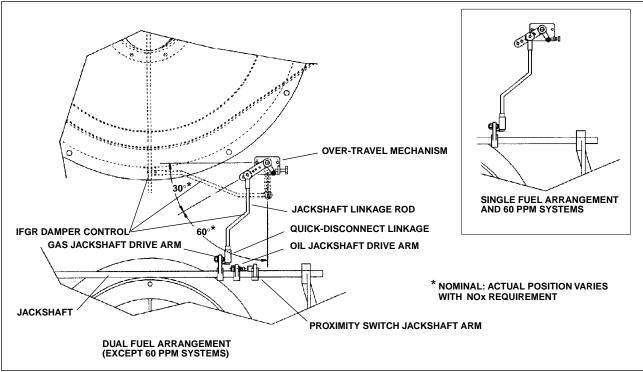
Figure 8-9: CB-LE Damper Linkage
