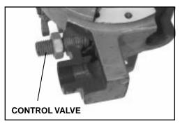
Figure: 5-6 Air Intake Control Valve
