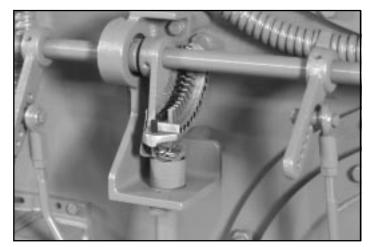
Figure: 2-13 Gas Modulating Cam
