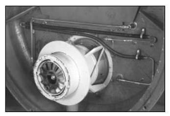
Figure 8-33: Inspect and Clean Inside Front Head and Components
