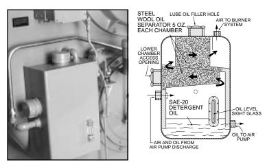
Figure 8-20: Air Oil Receiver Tank CB-LE
