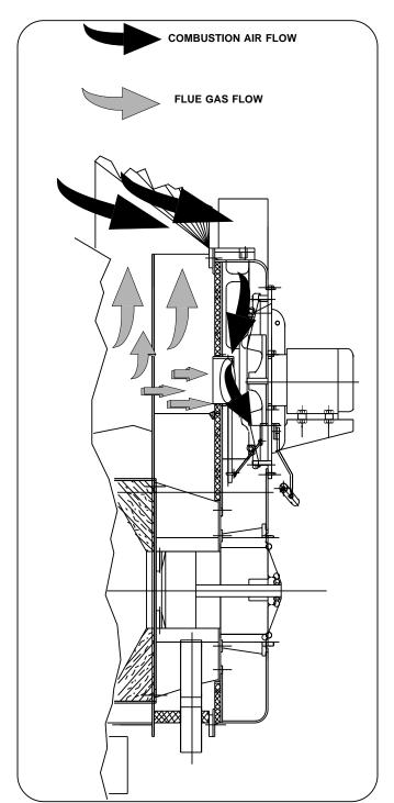
Figure 8-6: CB-LE Combustion Air and Flue Gas Flow
