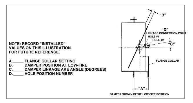
Figure 8-16: Flange Collar and Damper Settings (Top View)
