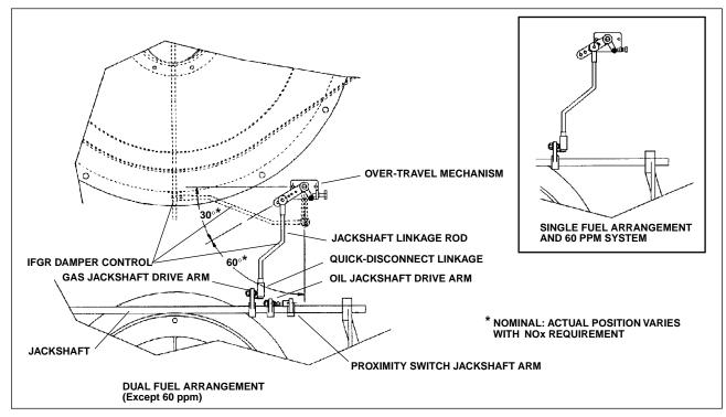
Figure: 1-16 IFGR Damper Linkage
