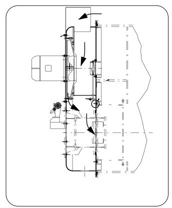
Figure: 2-24 Secondary Air Flow Diagram (CB-LE)
