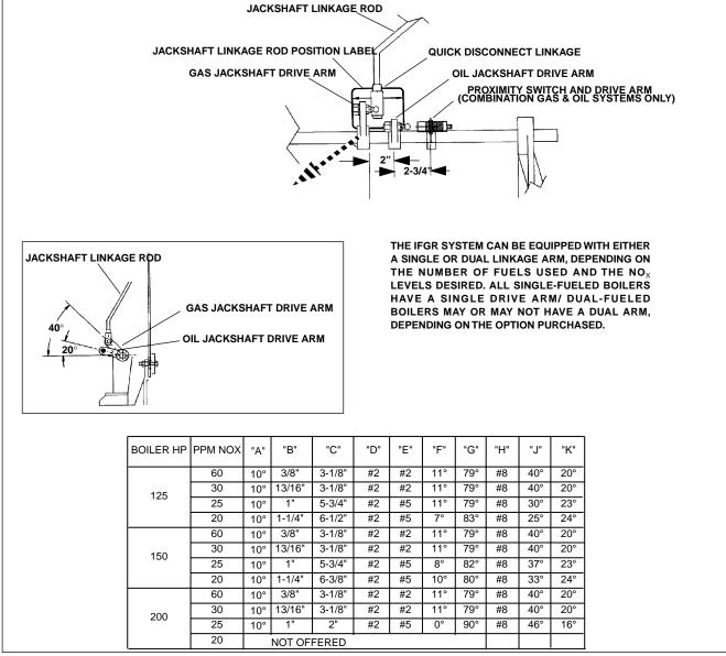
Figure 8-11: Jackshaft Linkage Settings
