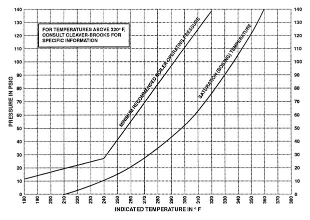
Figure: 3-3 Internal Boiler Pressure
