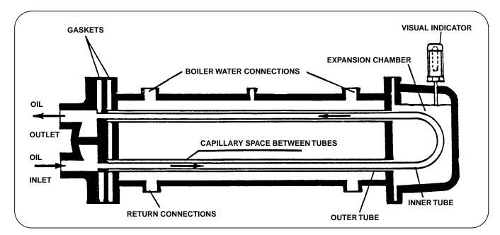
Figure 8-39: Circuit Layout of Hot Water Oil Heater
