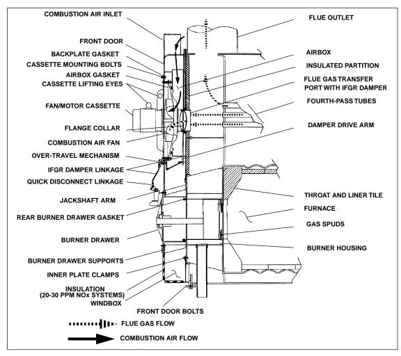
Figure: 1-15 Induced Flue Gas Recirculation System, General Arrangement
