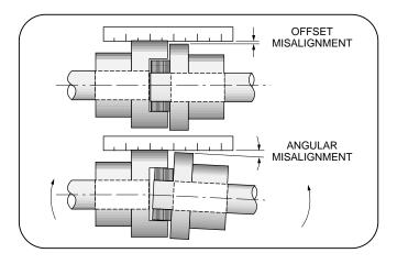
Figure 8-21: Coupling Alignment
