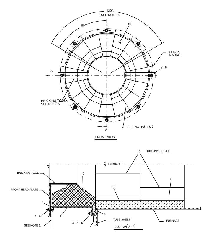
Furnace Liner & Bricking Model CB and CB-LE
