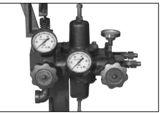
Figure: 5-12 Heavy Oil Fuel Controller
