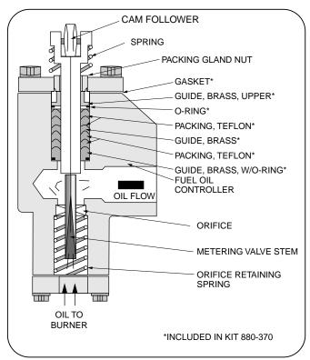
Figure 8-18: Metering Valve Packing Sequence
