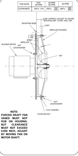
Figure 8-5: Forced Draft Fan Mounting
