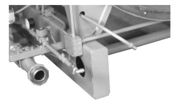
Figure 8-23: Disconnect Fuel lines and Sight Glass Cooling Tube.
