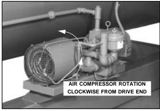
Figure: 5-2 Air Compressor CB-LE (CB Option)
