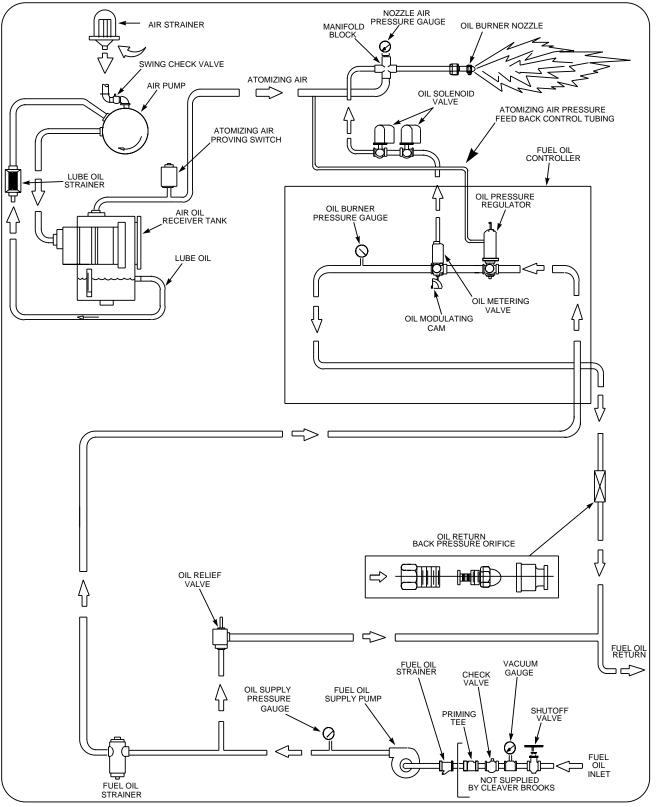
Figure: 2-25 Schematic Diagram for Light Oil Flow
