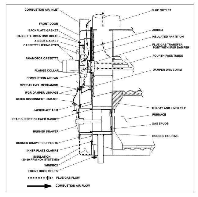
Figure 8-8: Induced Flue Gas Recirculation System, General Arrangement
