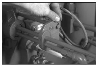
Figure: 5-13 Oil Gun Locked in OUT Position
