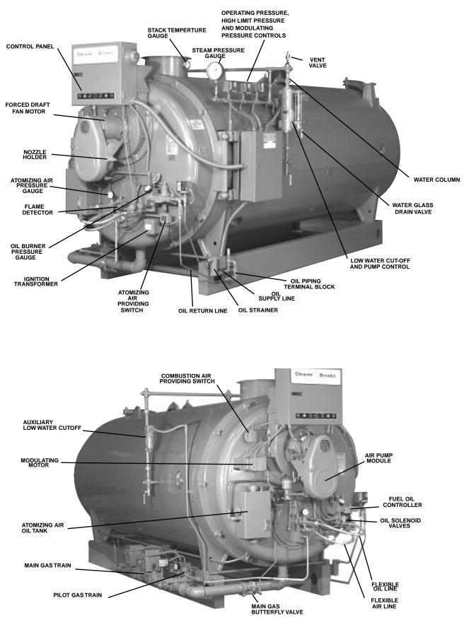
Figure: 1-2 Typical Steam Boiler - Light Oil or Gas Fired (CB)
