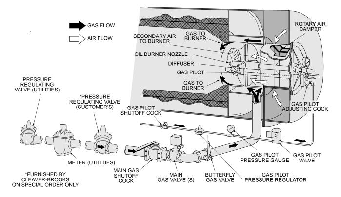
Figure: 2-15 Secondary Air Flow With Gas Train
