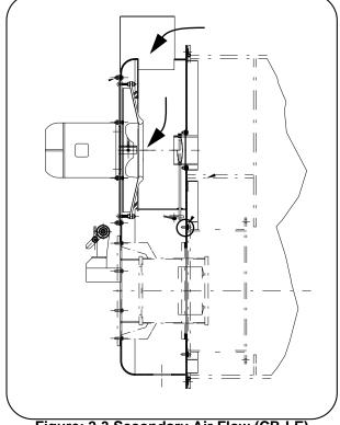
Figure: 2-3 Secondary Air Flow (CB-LE)
