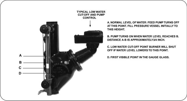
Figure: 3-2 Low Water Cut Off Sight Gauge
