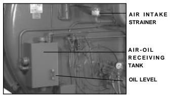
Figure: 5-5 Primary Air Strainer and Receiving Tank
