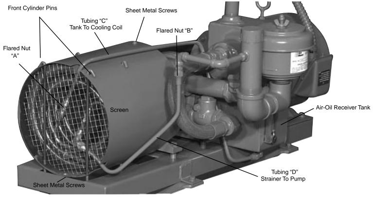
Figure 8-22: Side Mounted Air Compressor Details
