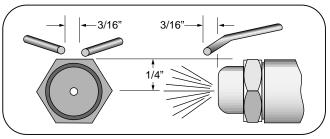
Figure: 6-14 Electrode Setting – Oil Pilot
