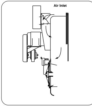
Figure: 2-2 Air Intake Through Front Head
