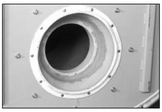
Figure 8-34: Fillet Dry Oven Contact Area
