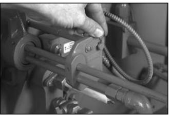
Figure: 6-18 Oil Gun Locked Out
