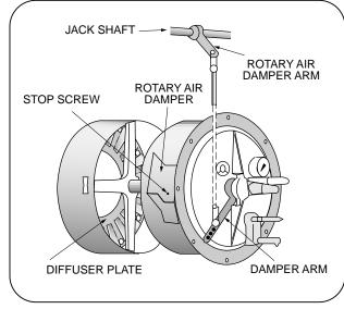
Figure: 6-2 Rotary Air Damper
