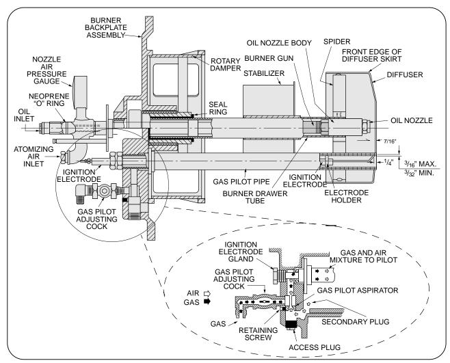
Figure: 6-15 Burner Drawer With Gas Pilot
